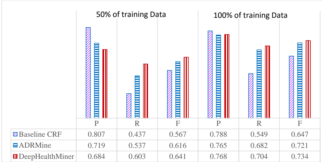
Figure 17: Impact of training set size on performance (precision (P), recall (R) and F-measure (F)) of different extraction methods (Twitter corpus).
