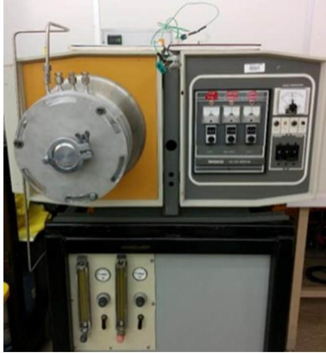
Fig. 15 A Mini-brute furnace for HT stress with N 2 and air flow.
