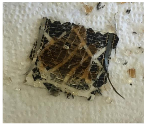
Figure 34: Removed Sample from TCE Solution
