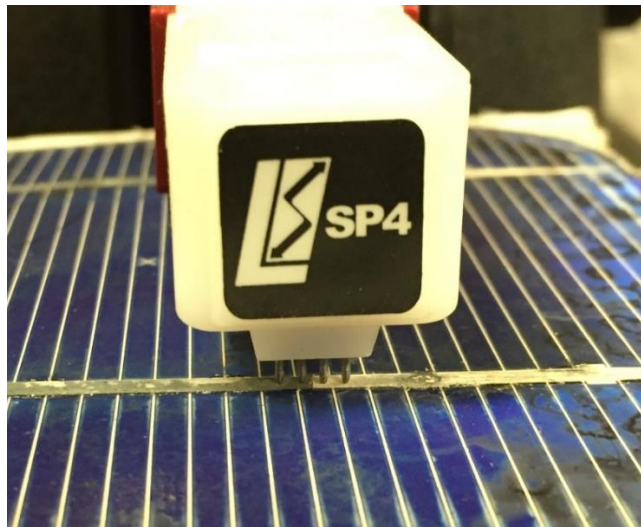
Figure 48: Placement of Four-Point Probe for Ribbon-Busbar Measurement
