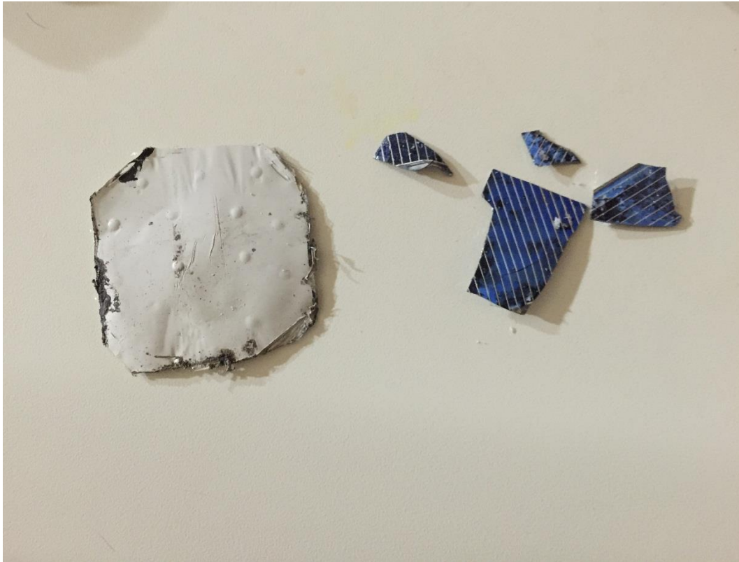
Figure 38: Separated Backsheet and Cell After Experiment
