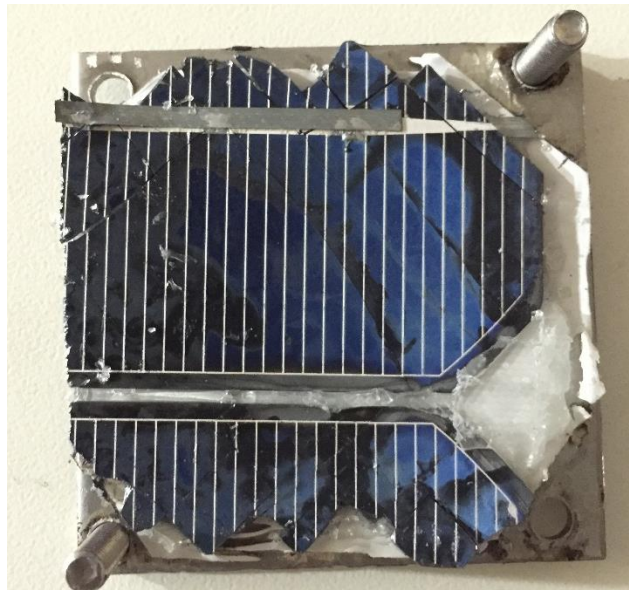
Figure 39: Sample After One Hour in TCE Solution
