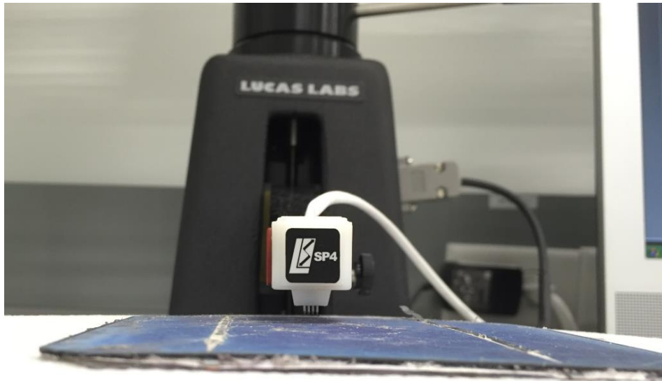
Figure 18: Four-Point Probe Setup Including the Probe and Keithley 2400 Multimeter
