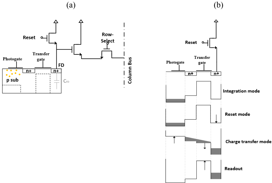
Figure 13 : (a) Schematic of photogate active pixel sensor (4T architecture) (b) Modes of operation of photogate
