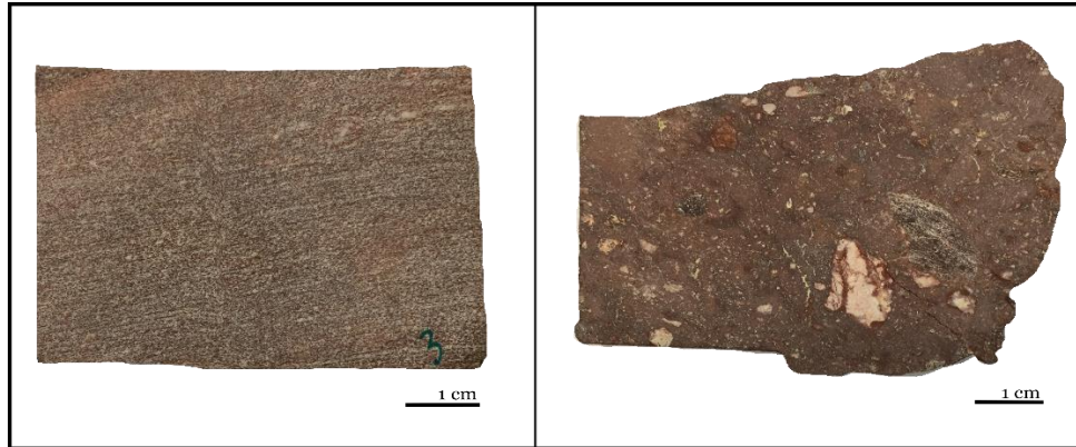
Figure 3: Hand sample photos of clast-poor (RIC_15_002, left) and clast-rich (RIC_15_015, right) samples of Montoume impactite.
