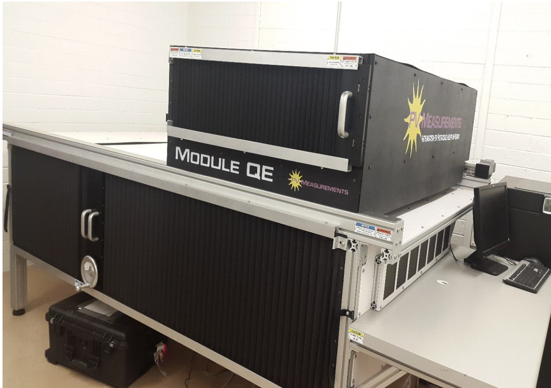
Figure 12: The PV Measurements QEX12M Machine Used to Measure the QE for the Samples- Before and After Soiling (Image Source:ASU-PRL)
