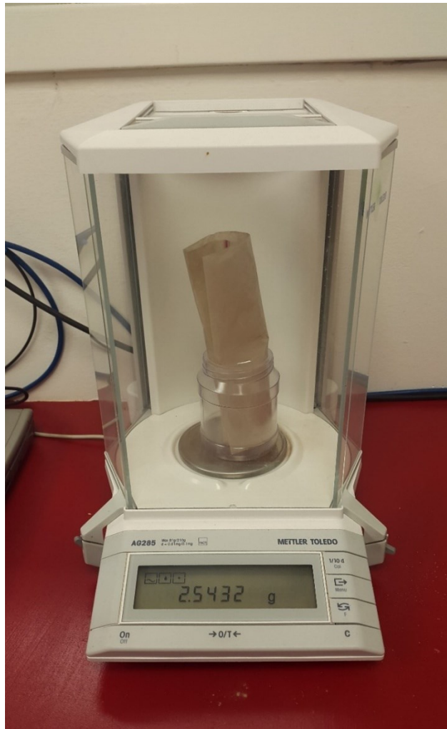
Figure 8: The Soil Collected in the Zip Lock Bag is Weighed (Image Source: ASU PRL)
