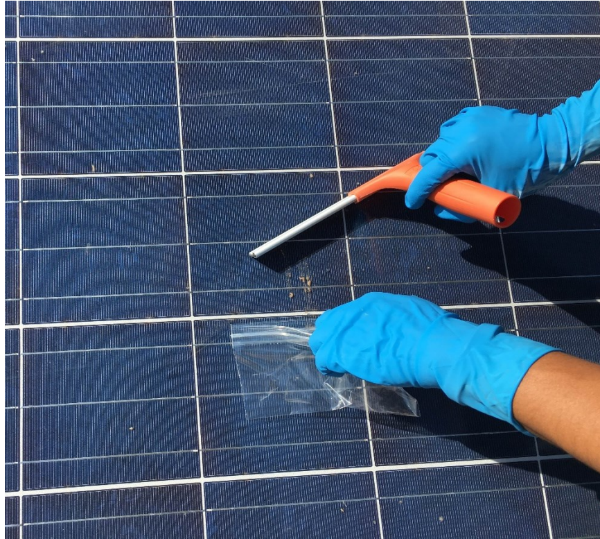
Figure 9: The Soil Collected from the Surface of the Module Using Squeegee and Zip lock Bag
