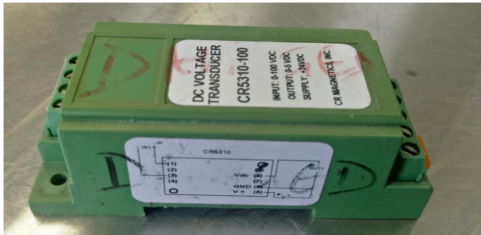
Figure 6: DC Voltage Transducer Used to Record Voc using Voltage Data Loggers
