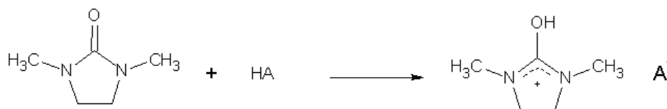
Figure 2-1. Protonation of DMI at its oxygen atom, developing a partial positive charge on nitrogen atoms and changing the C-O and C-N bond orders.
