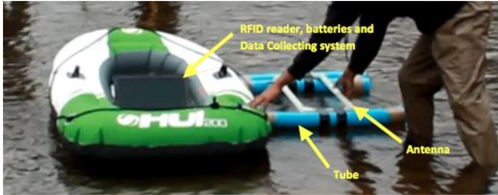
Figure 4.2 Installing the RFID System Near the Bridge Pier.
