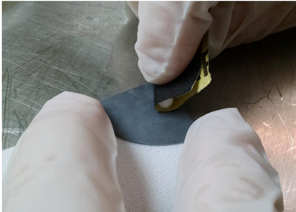
Figure A1. Backside of a GaSb wafer being roughened using 400 grit sandpaper wrapped around a cotton-tipped applicator.
