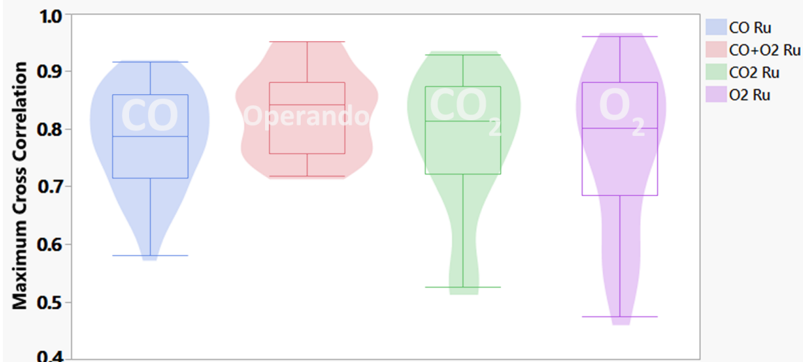
Figure 5-19 Shape Matching Cross Correlation Results Summary. Violin plot of the normalized cross-correlation with a more traditional box plot overlaid for each of the 3 in-situ conditions, as well as for the operando experiment. A cross correlation of 1 corresponds to a perfect match, which will never be achieved; >0.85 is considered a very good match, as discussed in Appendix IX.
