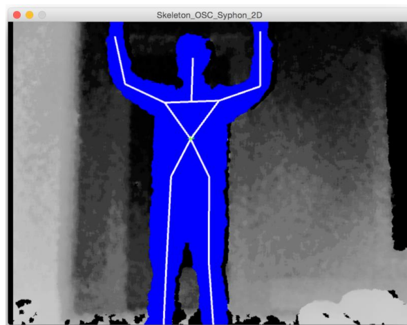
Figure 3.2. Skeleton Joint system from Microsoft Kinect
