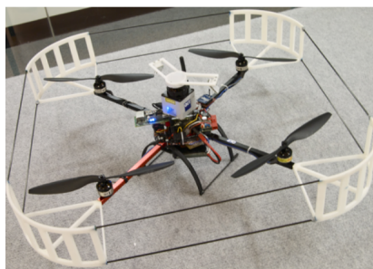
Figure 1.2: Quadrotor with Mounted Laser Scanner. © 2012 IEEE
