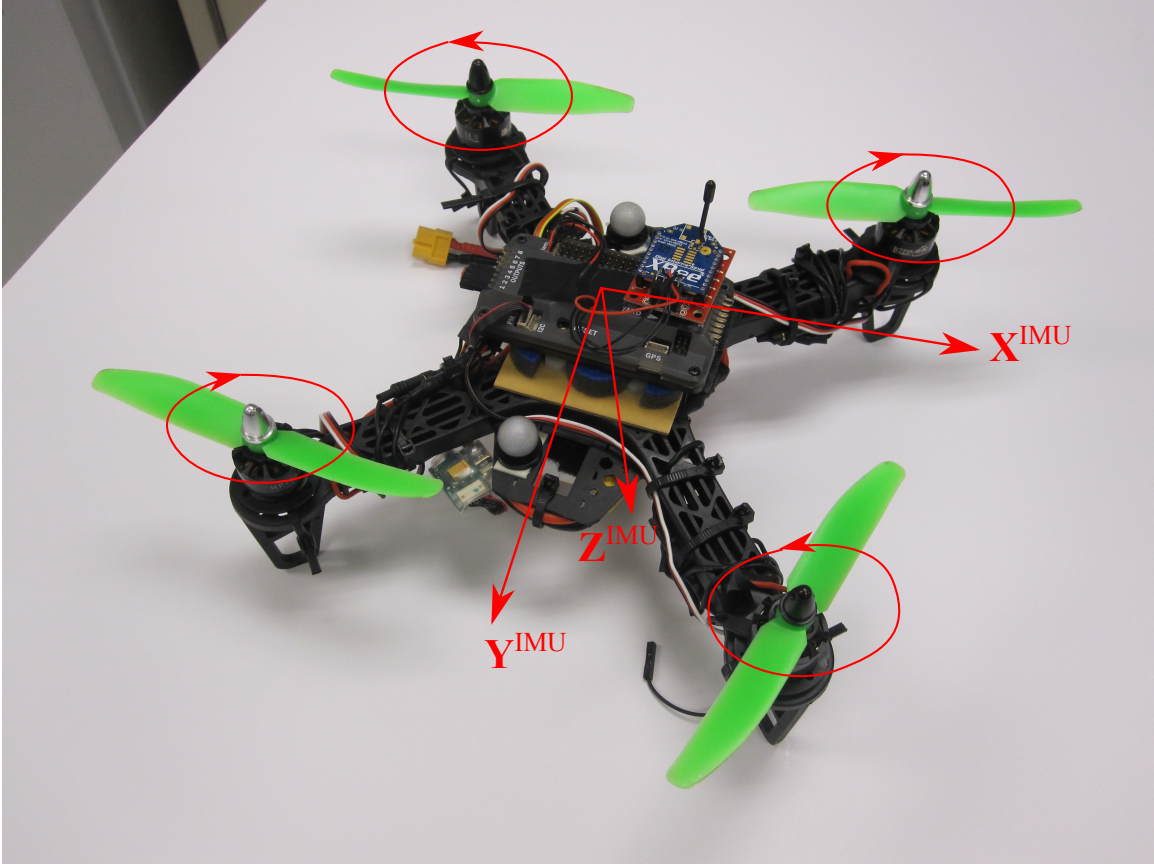
Figure 4.5: Coordinate System Utilized by Inertial Measurement Unit.
