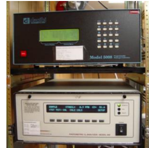
Figure 3.2 The photo above to the left is of the ADEQ JLG Supersite monitoring site in downtown Phoenix, and the photos above to the right show the stainless steel inlets where ambient air is drawn in and then analyzed in the ozone instrument below. While not all monitoring stations are set up in the same fashion, they all use the same equipment and adhere to certain siting regulations. (Photos courtesy of ADEQ).
