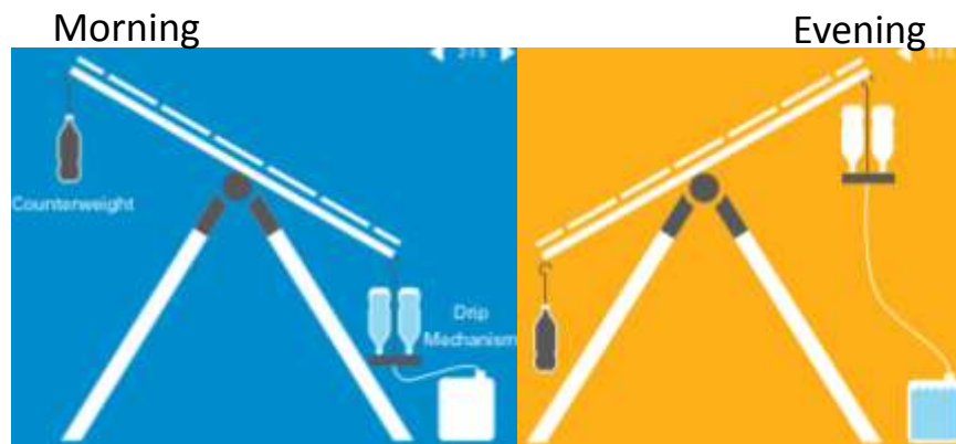
Figure 3: Schematic of the SunSaluter which utilizes weights that shift during the day to adjust the tilt of the solar panels. Potable water is a byproduct of this process. 9
