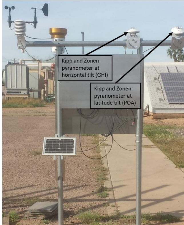
Fig. 12. Weather Station and Irradiance Sensors Used to Measure GHI and POA Irradiance ( 33^\circ South Facing Tilt) for 2013 and 2014 in Mesa, Arizona.
