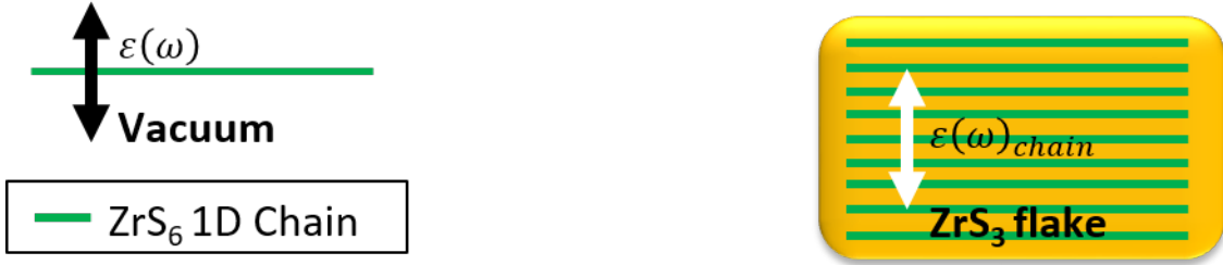
Figure 22. Left - Free standing 1D \text{ZrS}_3 chain. Right - 1D chains embedded in the matrix of \text{ZrS}_3
