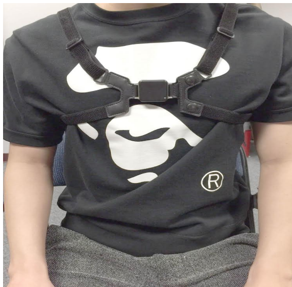
Figure 3.1 Participant Wear the Opal Sensor in the Center of Chest for Evaluation.
