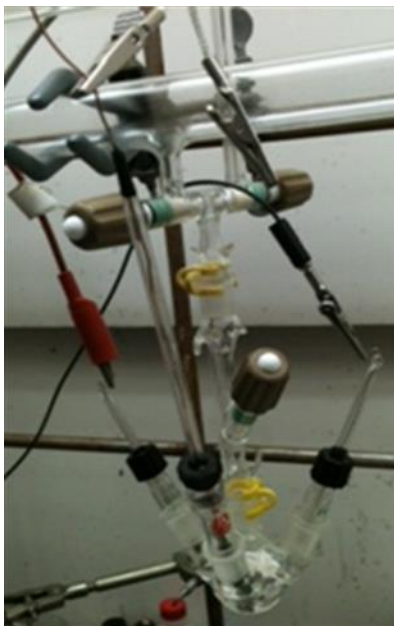
Figure 2: Picture of electrochemical cell set-up attached to the vacuum line. The cell consists of four necks, one for each electrode and one for connecting the cell to the vacuum line. Wires connecting the electrodes to the external circuit were sealed with leaded “flint” glass.
