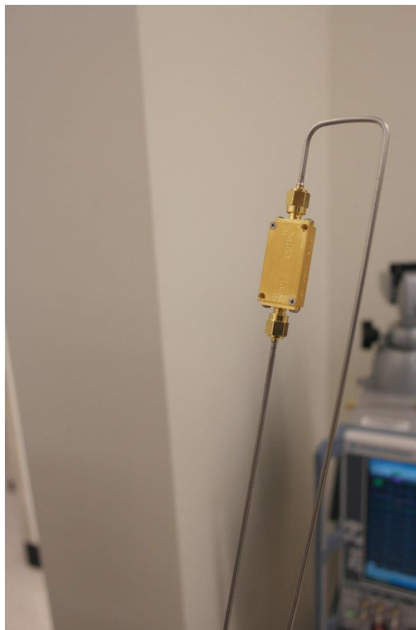
Figure 4.18 Dip probes attached to the microwave package housing the chip
