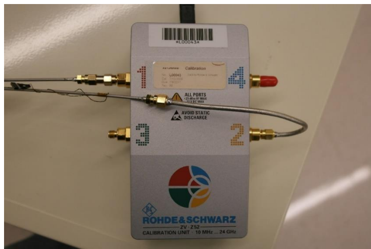
Figure 4.17 Calibration unit for calibrating the baseline transmission and reflection of the high frequency cables.
