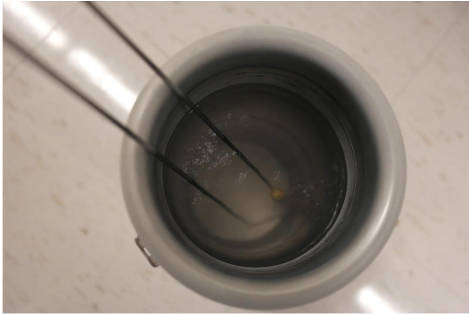
Figure 4.19 Package dipped in liquid nitrogen at 77 K
