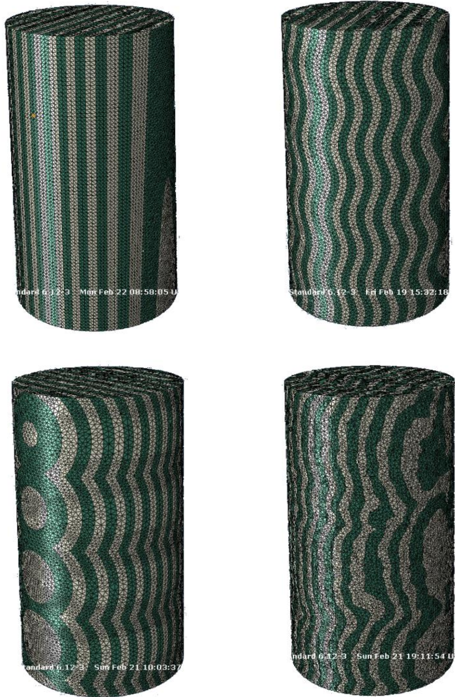
Figure 34: Pillar models used with flat, cosine, arc segment, and FIB derived nanostructures (respectively from left to right). Al layers are depicted in green while SiC layers are depicted in gray.
