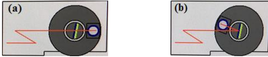
Fig. 19. Schematic diagrams showing optics arrangement in (a) transmission mode; (b) reflection mode
