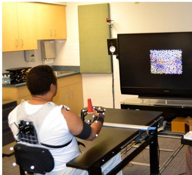
Figure 6: The stroke rehabilitation system [32], that uses a 14 marker configuration to provide feedback on motor function for stroke patients. A typical evaluation protocol requires a therapist to observe a specified movement to give a score indicating the quality of movement.
