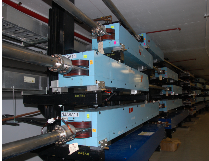
Figure 3.3: Bending arc magnets in the CEBAF accelerator. Each magnet bends electrons of a specific momentum for that particular recirculation.
