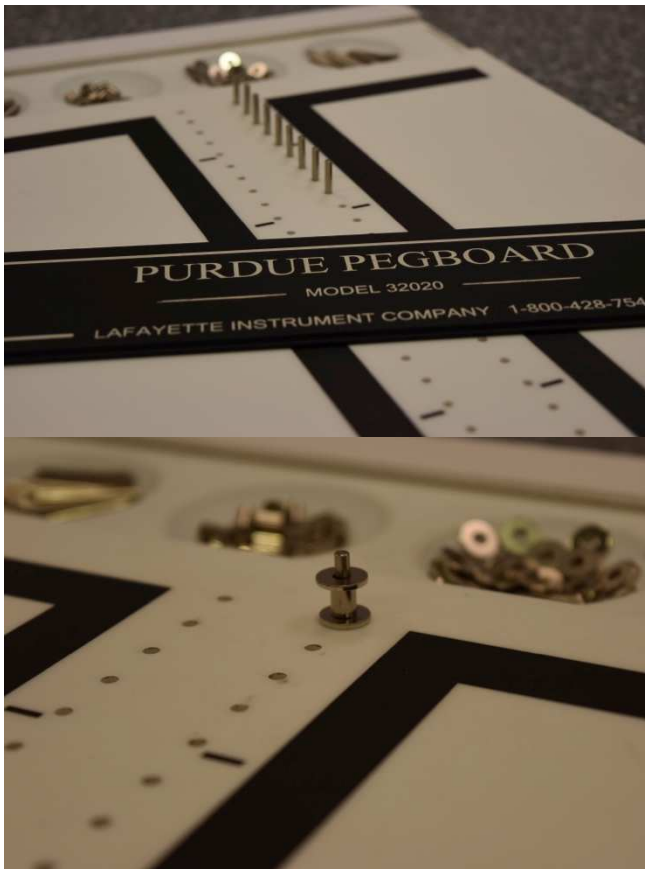
Figure 1: Purdue Pegboard with pegs for right hand dexterity test (top) and pieces for assembly test (bottom).
