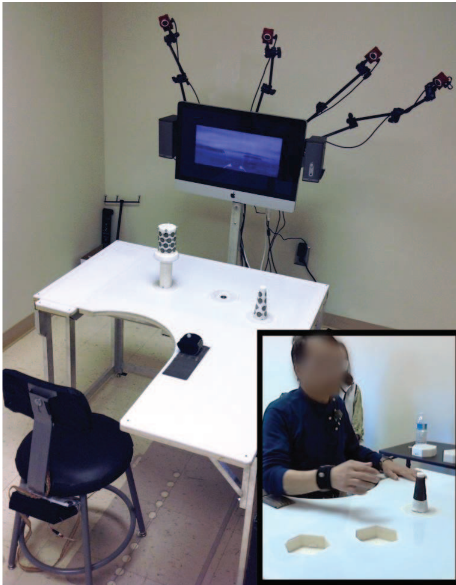
Figure 4.2: The Home-based Adaptive Mixed Reality Rehabilitation (HAMRR) system designed for stroke survivors. The system uses four OptiTrack cameras to track the wrist movements as well as a computer and speakers to provide audio and visual feedback during therapy treatment. The table is designed to accommodate custom touch and grasp objects for training reaches in different orientations. In the inset, we see the placement of a wrist marker on a participant performing reaching tasks to a cone. The system design is discussed in detail in [10].
