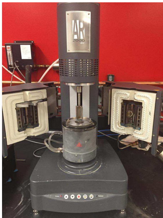
Figure 8: TA Instruments AR2000EX used in this Study, shown in Vane Geometry Configuration.
