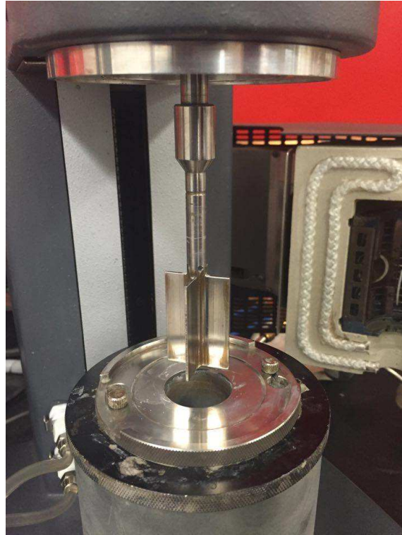
Figure 9: Cup-and-bob Geometries used in Study
