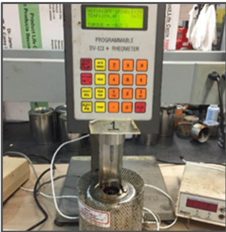
Figure 2-6: Brookfield Device placing a spindle in the tube heat chamber
