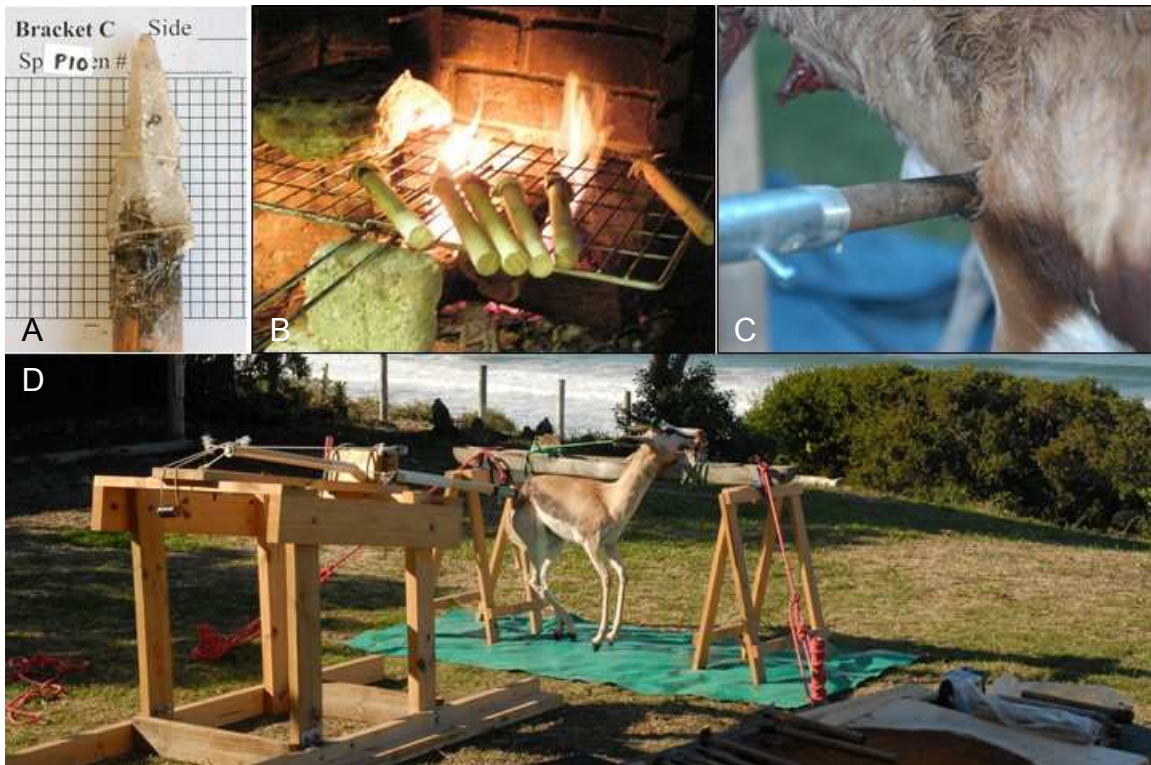
Figure 19. Spear armature setup. A) Quartzite point hafted. B) Points drying in kiln. C) Point lodged in carcass after being fired. D) Calibrated crossbow setup.
