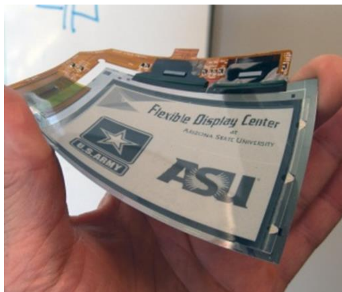
Figure 1.11: Flexible Display Produced on 125 \mu\text{m} Thick Stainless Steel Foil
