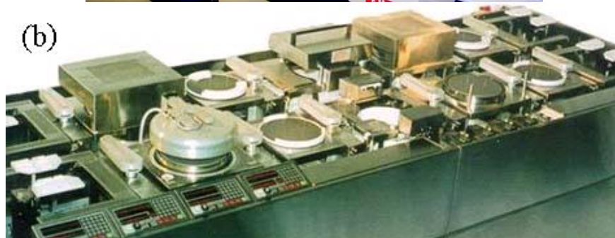
Figure 1.14: Images of (a) Automated Batch Processing Wet Etch Hood and (b) Photoresist Coater and Developer Track
