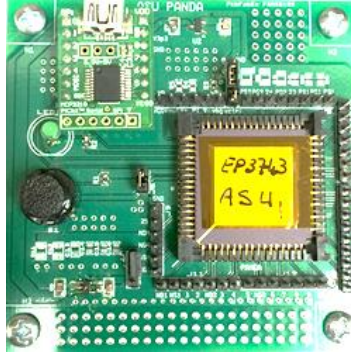
Figure 4.2. Test board consisting of PANDA chip in a socket, an add-on board with MCP2210 for reconfiguration and other components for flexibility in measurements.
