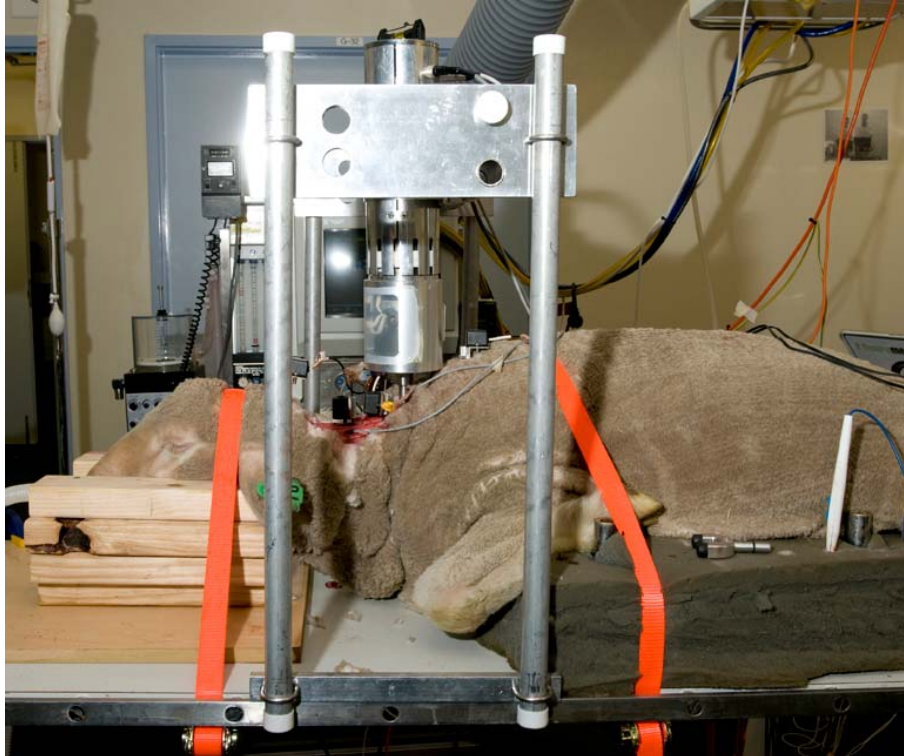
Figure 14. Experimental setup showing positioning of the biomechanical testing apparatus, fixed frame, and tri-axial accelerometer placement.
