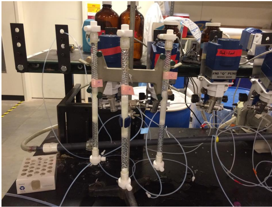
Figure 2.3: SBG-1 Packed Columns for Treatment of SRP Groundwaters.
