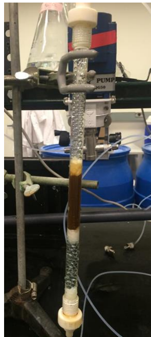
Figure 2.2: Bayoxide E33 Packed Column for Treatment of SRP Groundwater Wells SBG-1 column operation
