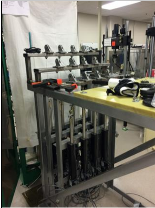
Figure 6: 12 Actuator Set-Up of Upper Extremity Feedback Controller
