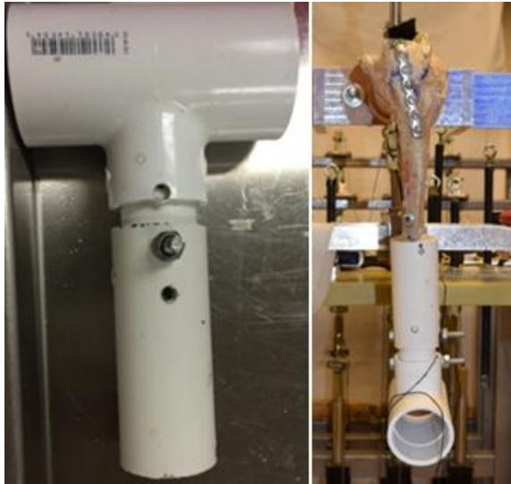
Figure 15: Distal Fixture to Accommodate the Length of Lost Forearm and Hand Formed Using Anthropometric Data
