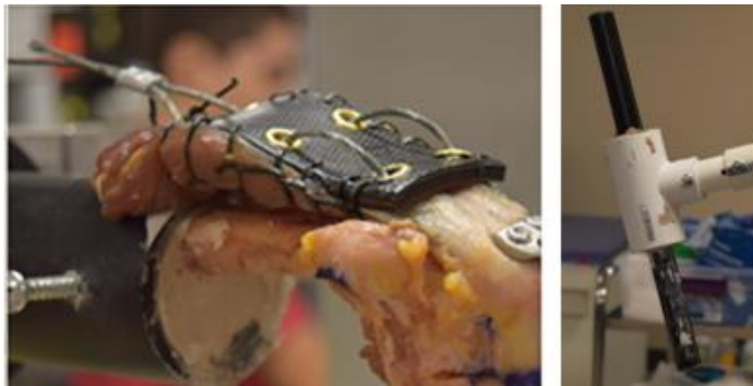
Figure 41: Improved Suturing Technique at the Triceps Tendon, Leather Belt Strap was Used with Two Rows of Rivets to Attach with Steel Cable; T-Shape Potted with Dumbbell Rod
