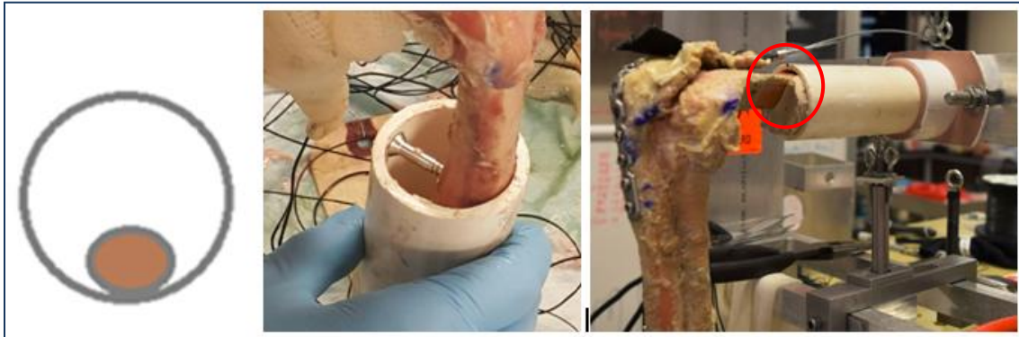
Figure 36: Potting Technique of Humerus was Improved By Potting it at the Edge of The Fixture which in Turn Reduced the Insertion Angle
