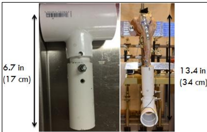
Figure 27: Designed Distal Fixture to Compensate the Dissected Ulna-Radius Bone and Hand
