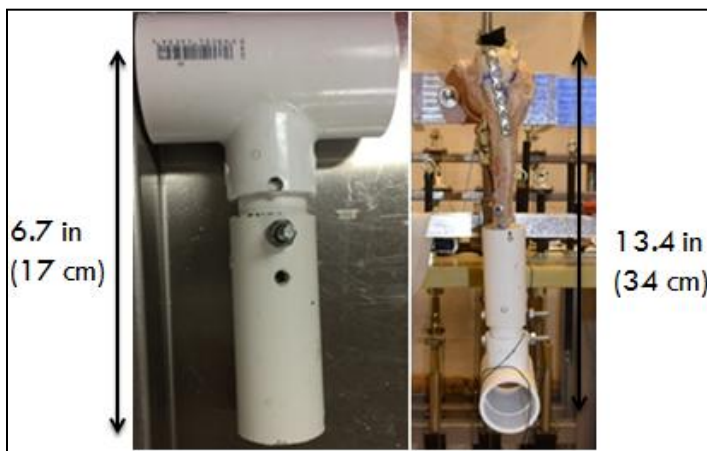
Figure 38: Distal Fixture Created after Anthropometric Calculations of the Length of the Forearm and Hand of 16 Cadaveric Specimens from the Cadaveric Database
