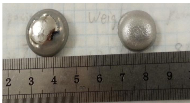
Figure 3.2 Alloy buttons after arc melting. Button on the left is \text{Ni}_{60}\text{Nb}_{35}\text{Zr}_5 , button on the right is \text{Ni}_{60}\text{Nb}_{35}\text{Sn}_5
