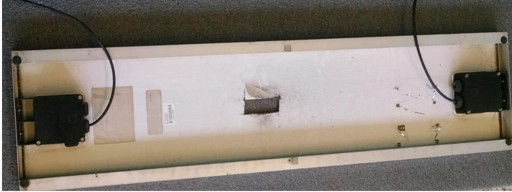
Figure 32: Photograph of a Module With Center Part of a Cell Removed from the Laminate
