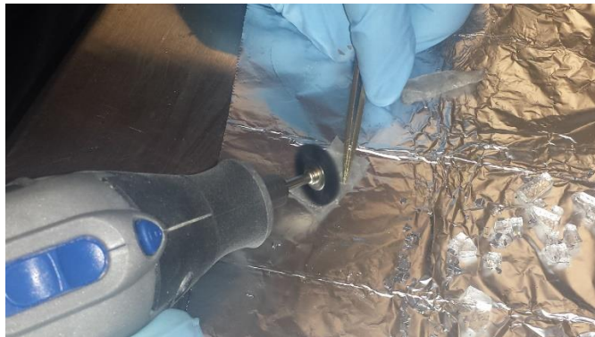
Figure 31: Dremel Tool Plastic Brush Cleaning the Extracted EVA layer
