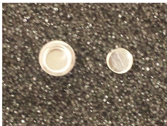
Figure 35: Hermetically Sealed pan (left) with its Lid (right)
