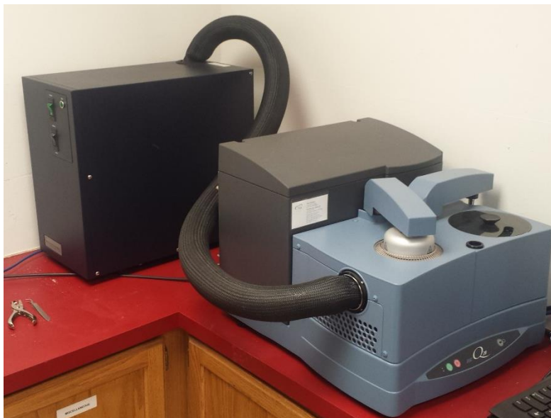
Figure 34: DSC and Cooling Tower Attachment Used for DSC Analysis
