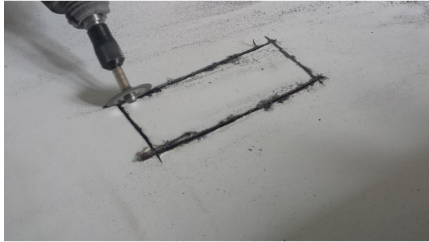
Figure 30: Diamond Dremel Tool Cutting Out the Center Part of a Cell
