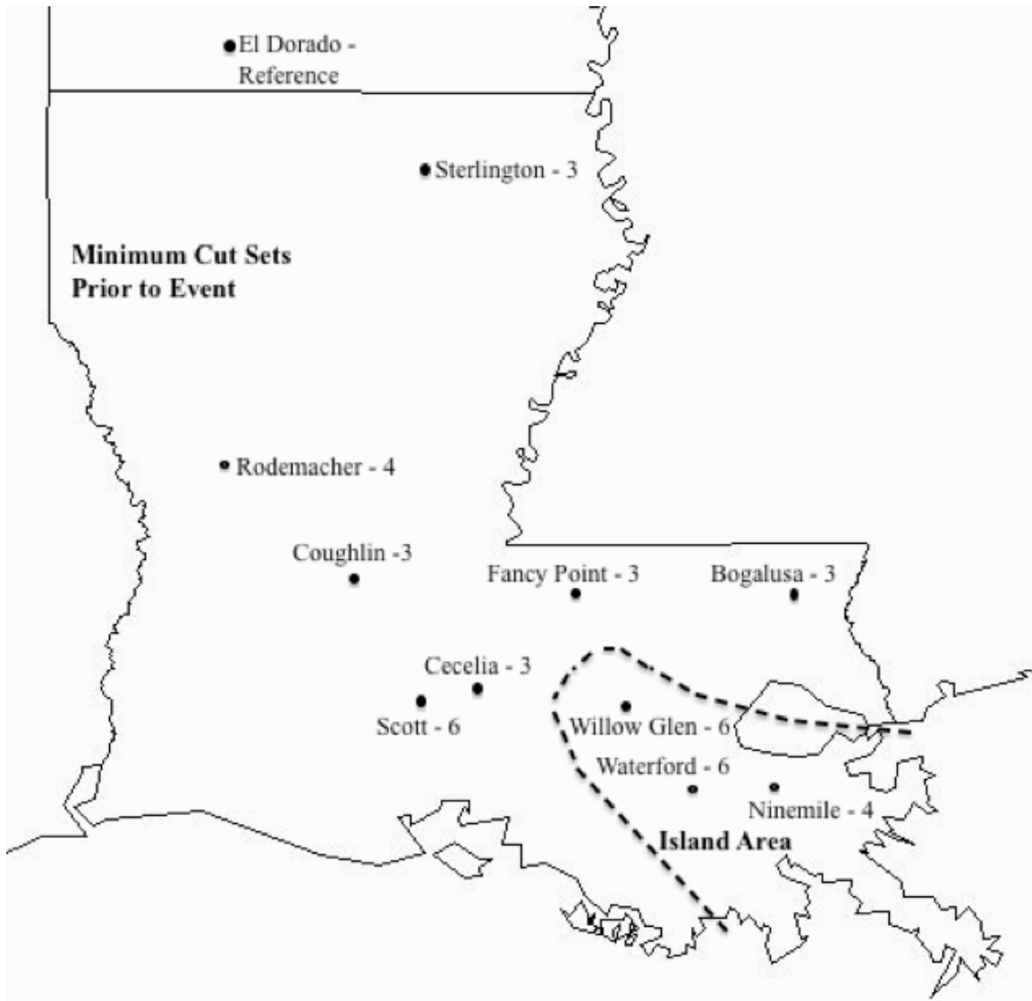
Fig. 2.4 The Maximum Flow to Selected Sinks Within the Entergy System Prior to the Event.
