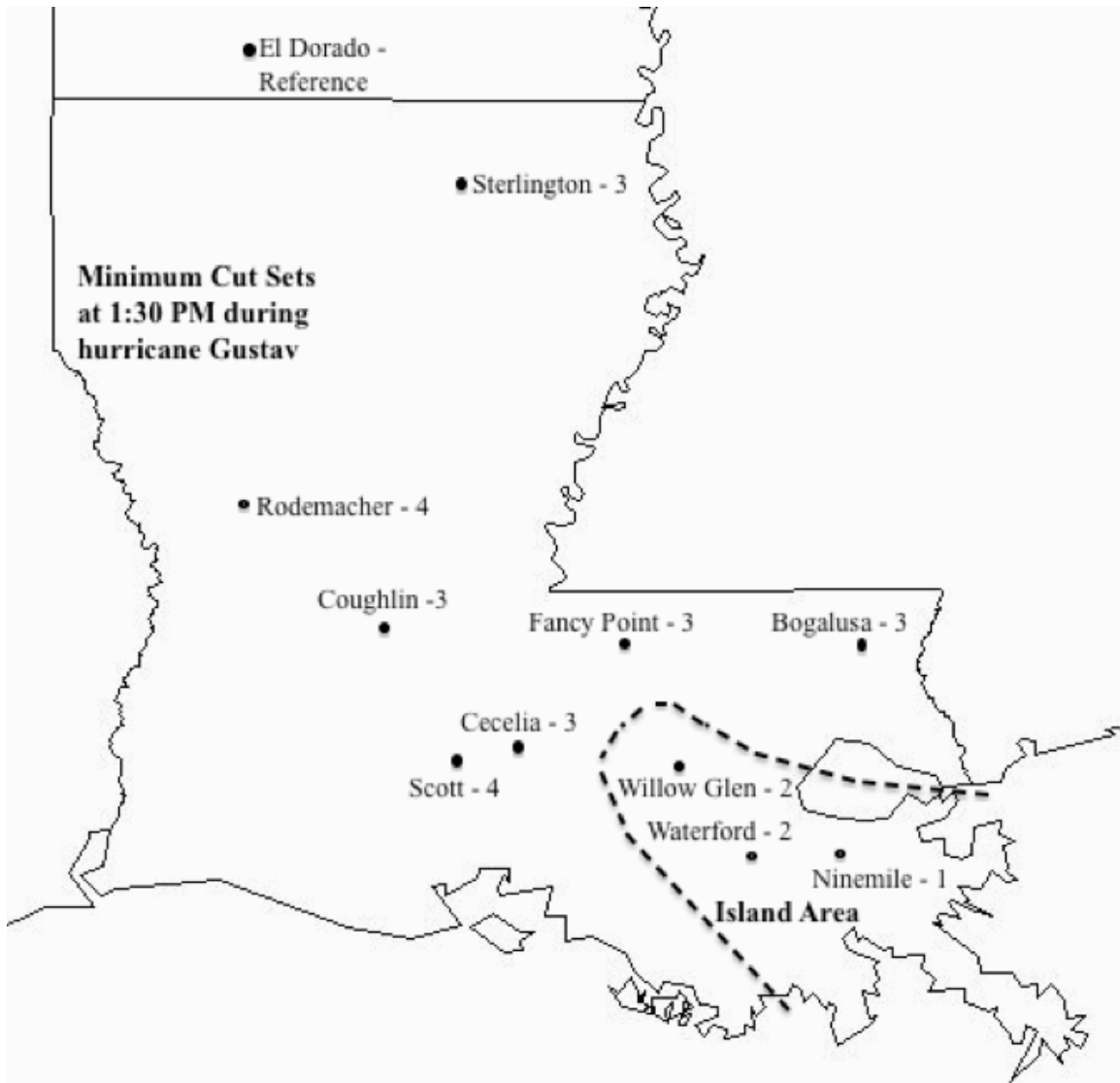
Fig. 2.5 The Maximum Flows to Selected Sinks Within the Entergy System at Approximately 1:30 PM During Hurricane Gustav
