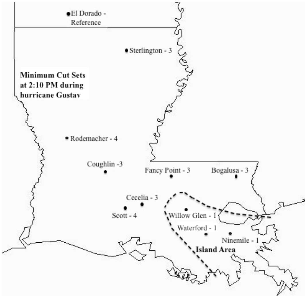
Fig. 2.6 The Maximum Flows to Selected Sinks Within the Entergy System at Approximately 2:10 PM During Hurricane Gustav
