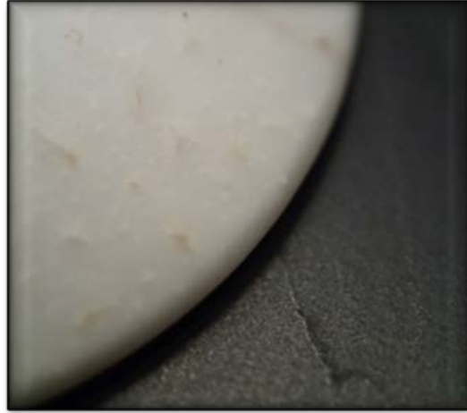
B. 0% opaque PLA after composting
