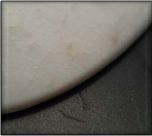
C. 2% opaque PLA after composting
