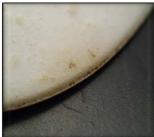
D. 10% opaque PLA after composting
