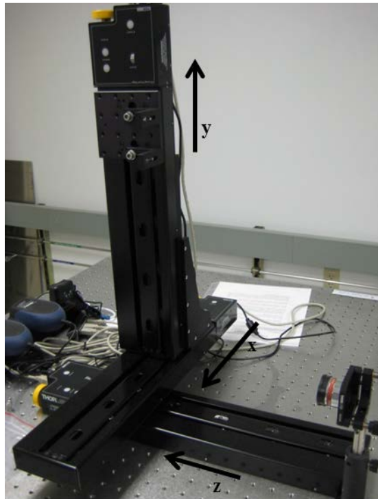
Figure 45: 3D automated stage setup showing x,y and z axis.
