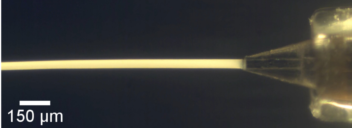
Figure 49: PEG 8 \times 10^6 in water solution at 7% concentration containing no sample and extruding in vacuum with a 50- \mu\text{m} inner diameter capillary.
