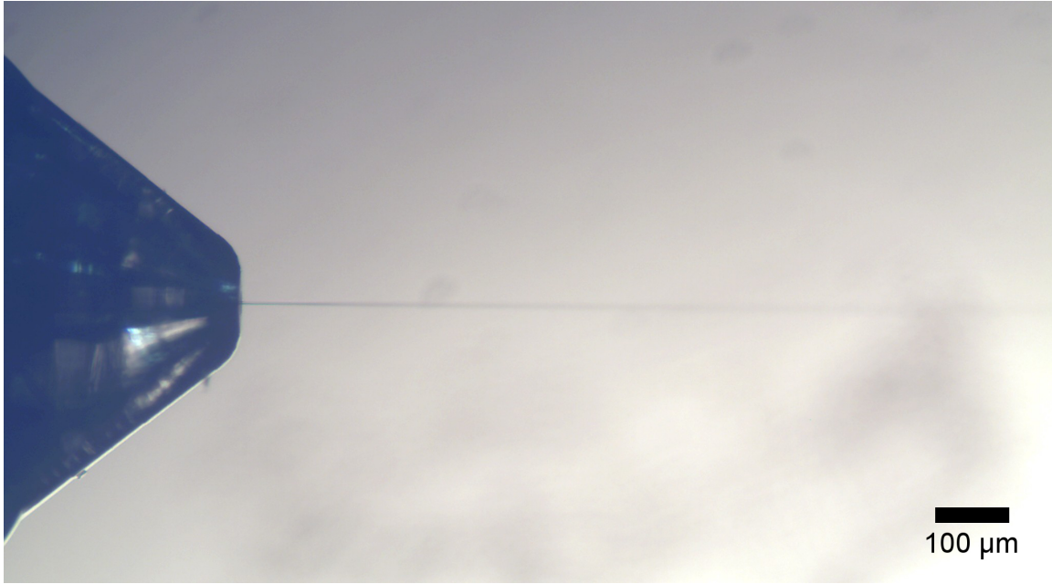
Figure 38: Improved prototype 2 nozzle with a straight jetting profile. No variation in angle was observed when rotating the nozzle.
