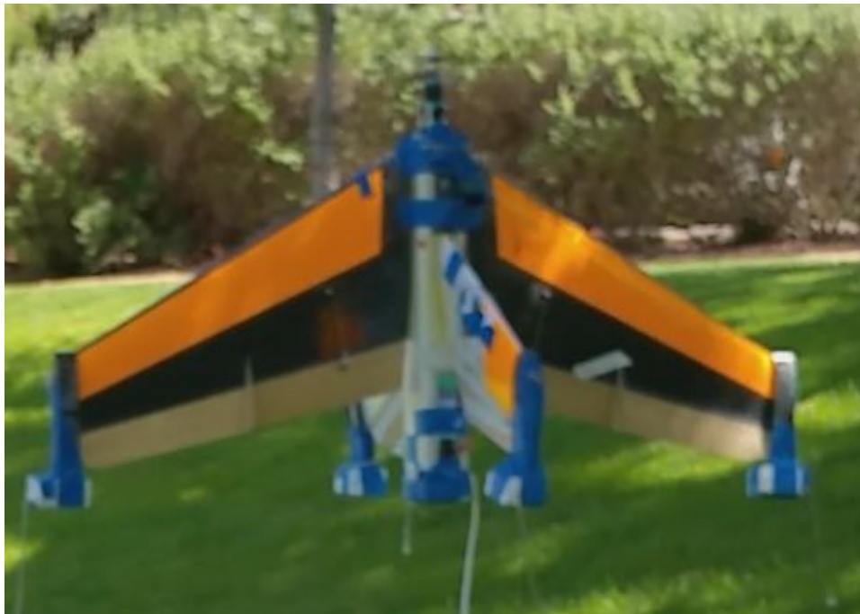
Figure 6. A picture of the VTOL drone we studied in this project in hovering state
