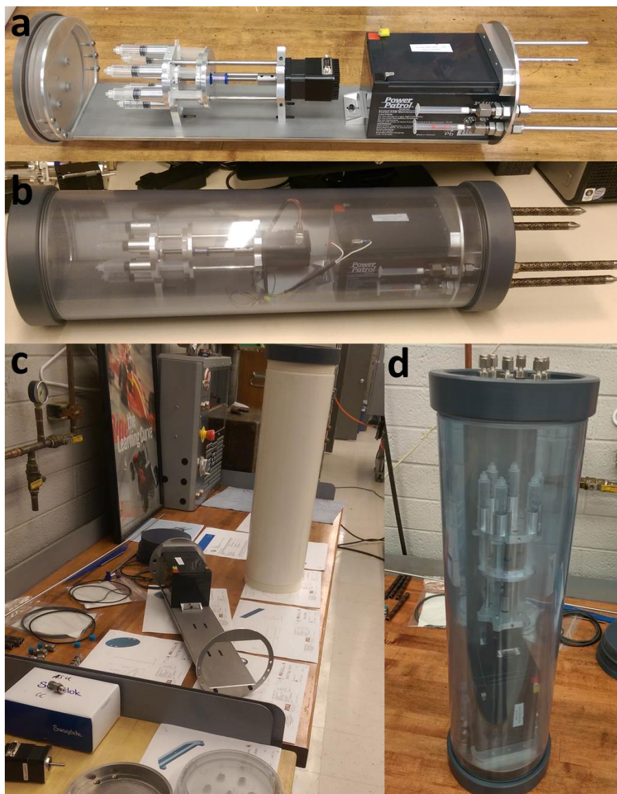
Figure 5-2. Pictures showing the internal components (panel a), including the syringes, pump motor, battery, and pore water extraction cartridges. Panel b shows the completed construction with a clear PVC shell. Panel c shows several individual components, including (from bottom to top) the stainless steel bottom cap, acrylic top cap, step motor, interior chassis, O-rings, battery, and shell. Panel d shows the constructed top tap with Swagelok fittings (for bulk water intake).
