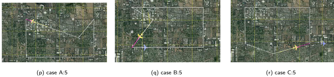
Figure 8.14: Path generation to simultaneously avoid two aircraft for greedy closed-loop RRT. The green icon is the UAV and the blue is the obstacle aircraft. The white cross indicates the predicted collision location. In each column, encounters happen in different sections of the original flight plan. Each column shows a different situation. Collisions of the two aircraft with the UAV happen closely in the UAV's original route in each case.
