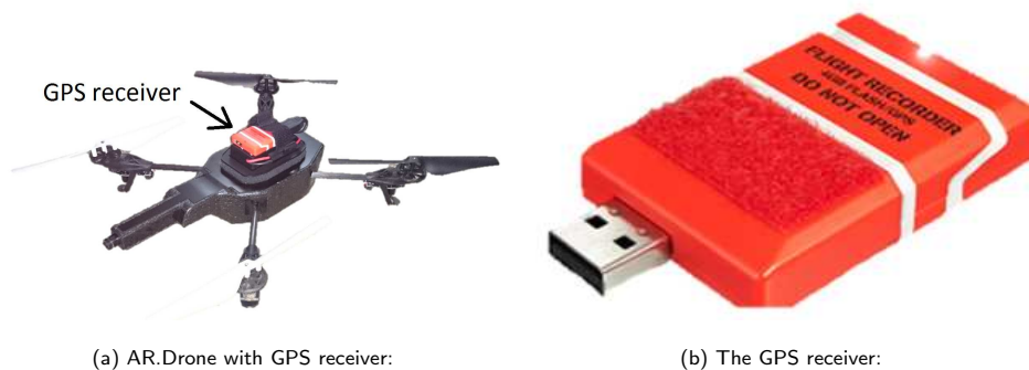
Figure 3.16: The AR.Drone used in the real flight experiments 3.16a and the GPS receiver attached to it 3.16b.
