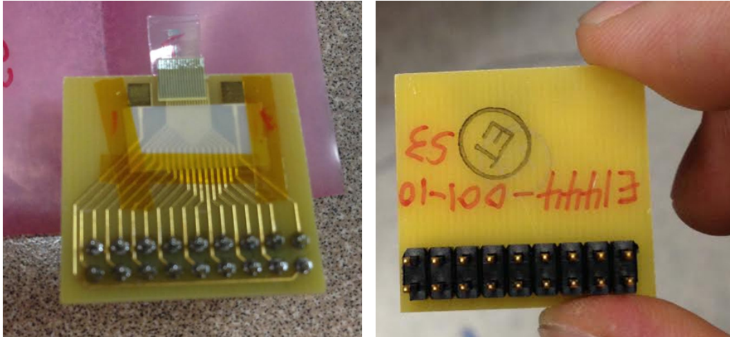
Figure 26: Top view (left) and bottom view (right) of an InGaZnO TFT preamplifier bonded to a pinout PCB.
