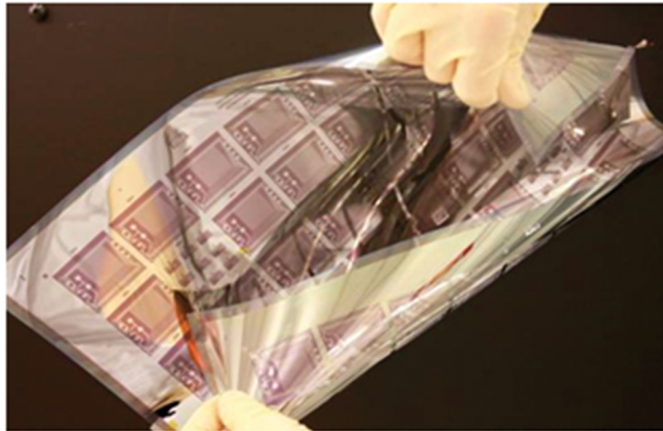
Figure 7: Photographs of a wafer of flexible electronics (left) and a flexible display (right) built at FEDC.
