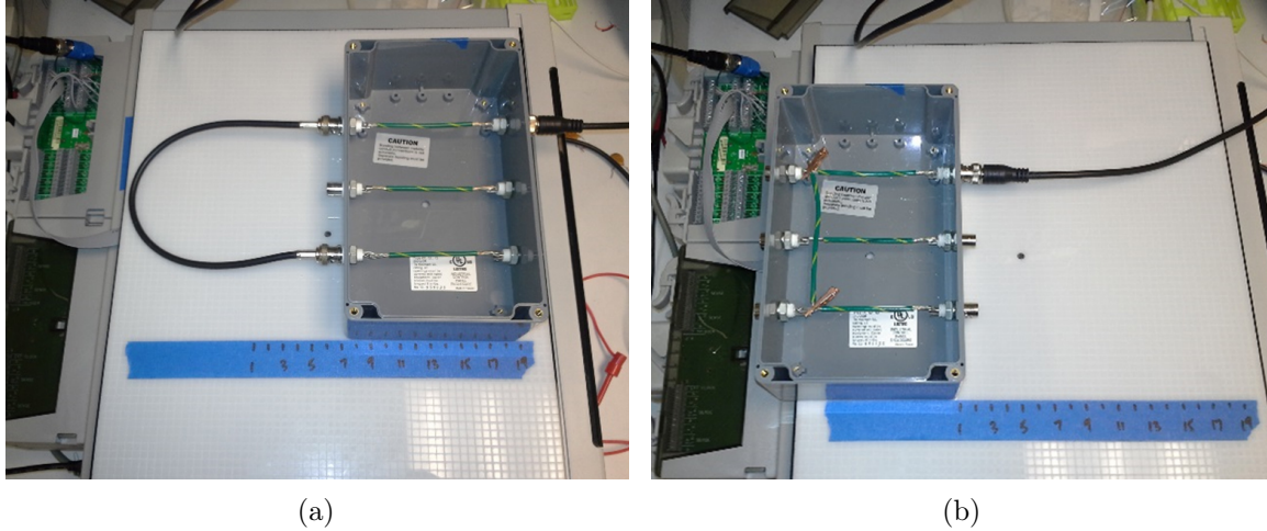
Figure 59: (a) Setup 1: Experimental setup of a plastic box with 3 parallel wires. (b) Setup 2: similar setup but in which the top and bottom wires are connected with a jumper wire within the box.
