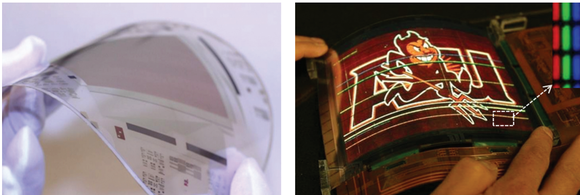
Figure 6: Photographs of a wafer of flexible electronics (left) and a flexible display (right) built at FEDC.
