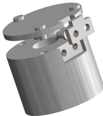
Figure 7: Cap cylinder assembly CAD model
