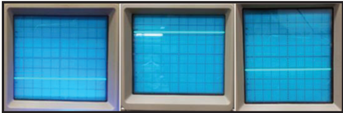
Figure 4.12 Optoscope Reading: Left: Baseline, Middle: Direct coupling of led, Right: led coupled to the Optical System
