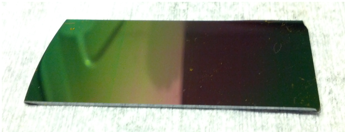
Figure 47 – Sample deposited at a high chuck speed after a nozzle clean
