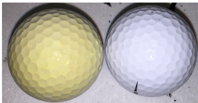
Figure 54 – Uniform deposition over the top hemisphere of a golf ball; proving Deppy’s ability to coat uniquely shaped and nontraditional objects.
