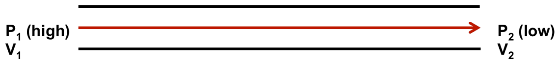
Figure 14 – Fluid flow through a constant diameter pipe. The velocity of the fluid will be dependent on the pressure drop as described by the Bernoulli equation
