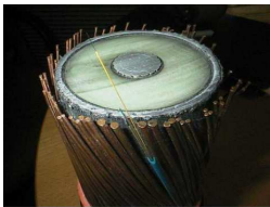
Fig. 2-5 Fiber Optic Embedded XLPE Cable [17].
