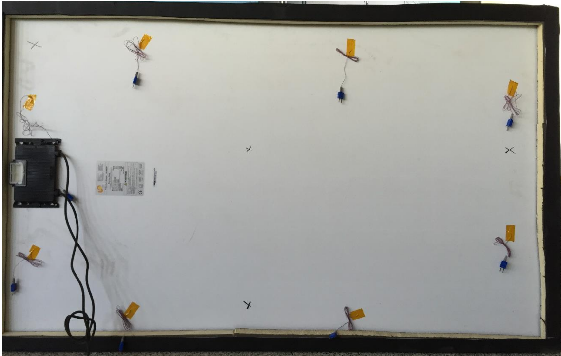
Figure 13. Frame insulated module with sensors on edge cells
