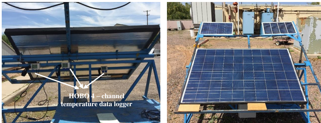
Figure 14. Module with frame and backsheet insulation - front and back view
