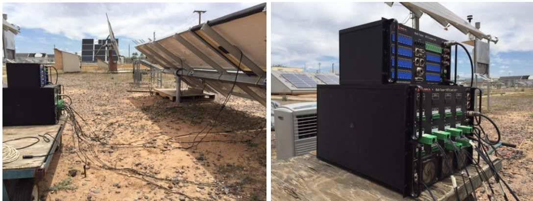
Figure 19. Modules connected to a multitracer – Monitoring temperature at Pmax
