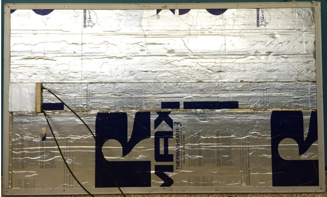
Figure 9. Module with back surface insulation
