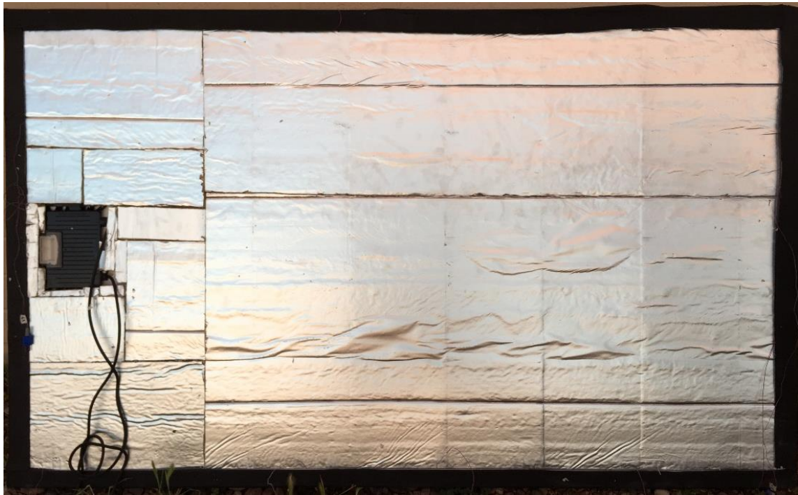
Figure 10. Module with frame and back surface insulation
