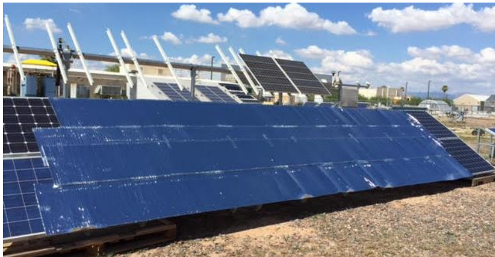
Figure 20. Modules shaded for temperature coefficient measurements
