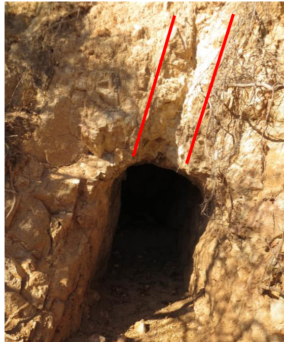
Figure 4.26. Adit located along El Tesoro trend showing mineralization (outlined in red) with a southeast dip of 67°. Adit opening is 1m in width.
